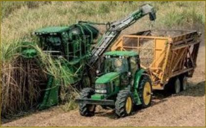
Mechanized Harvester feeding cane into 10+ MT trailer/tender
