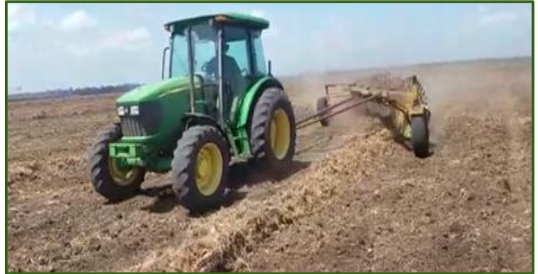
Mechanical rake quickly removes large amounts of smaller debris
