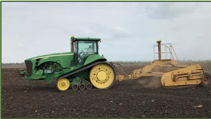
Heavy Tractor pulls GPS & Laser guided contour leveler
