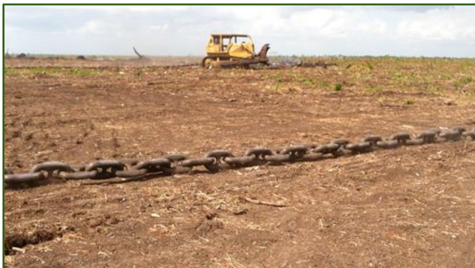
Side view of 150m long chain – each 60cm link weighs over 40 Kg
